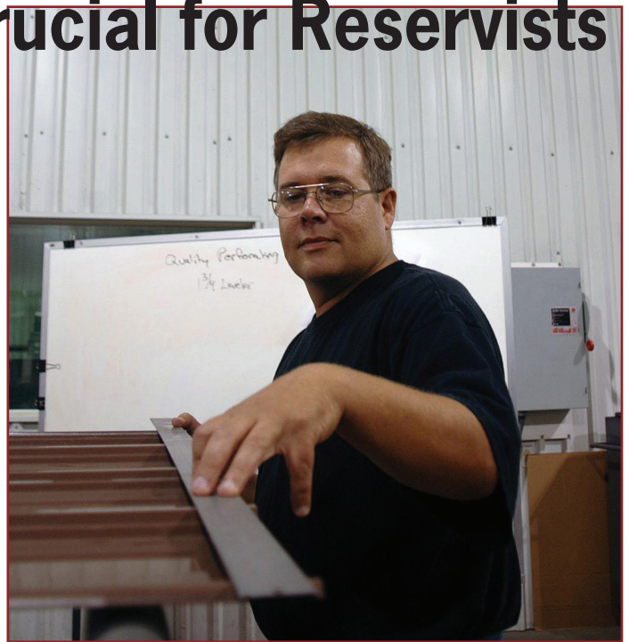
Sergeant Lofton measures a recently formed sheet of metal roofing.
