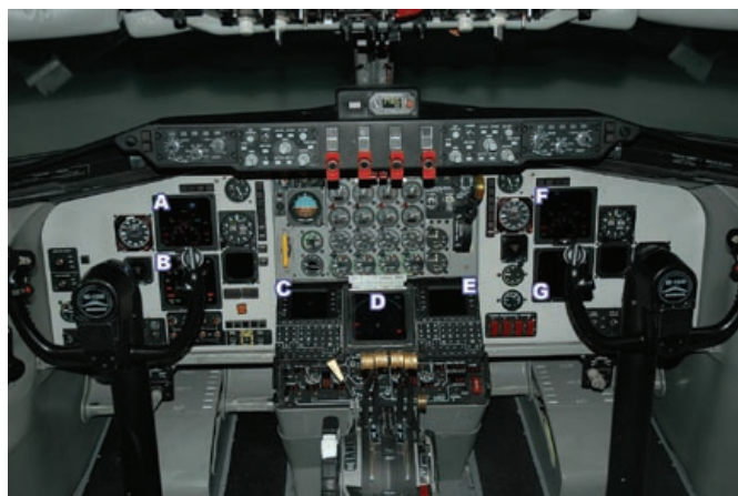
A & F: Primary Attitude Indicators. Both were locked at level. These normally show when the aircraft climbs or turns.
